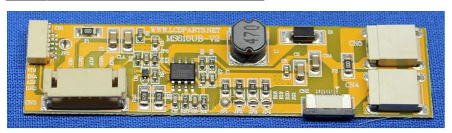
There two 6 pin connectors on MS610UB (CN1 and CN3). Their pin out is not the same (Printed on components side).
